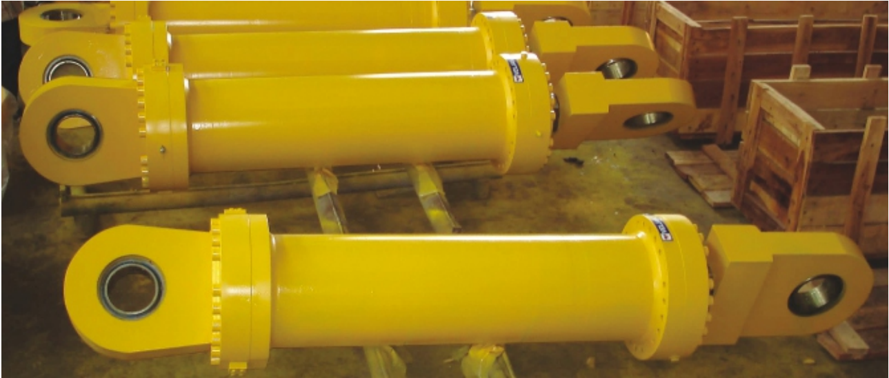
8. Typical View of packing of bore 360mm \varnothing x 200mm Piston Rod x 1500mm Stroke Stacker Reclaimer Hydraulic Cylinders (Operating Pressure 250 Bar Test Pressure 375 bar)
