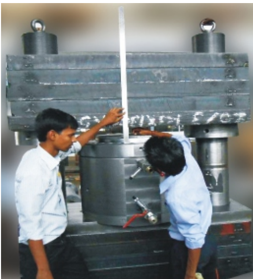
6, 7. Typical Views of Pressure testing facility for Roll Force Cylinders and Heavy duty Press Cylinders.
