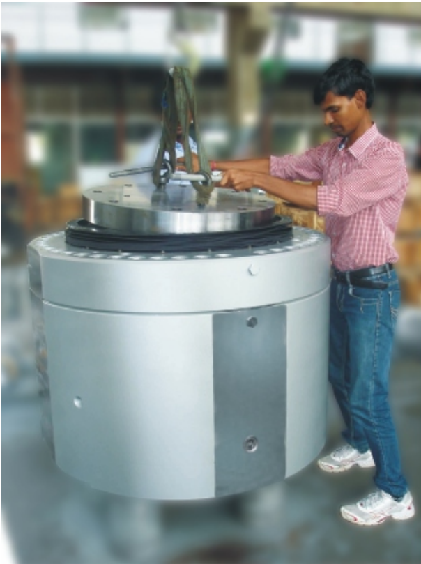
3. Typical View of a Roll Force Cylinders Bore \phi 800mm x Piston Rod \phi 750mm x Stroke 272.5mm --Fixing of Pressure Pad (Rocker Plate)
